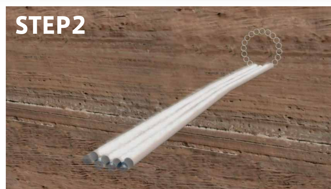
Making connections by RC structure between all the two shields
