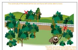
Figure 4.2: Example of the barrier effect (Source: [5])
