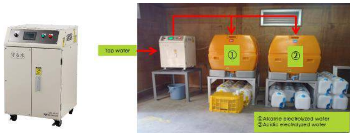
Figure 2: Production of alkaline water and acidic water
