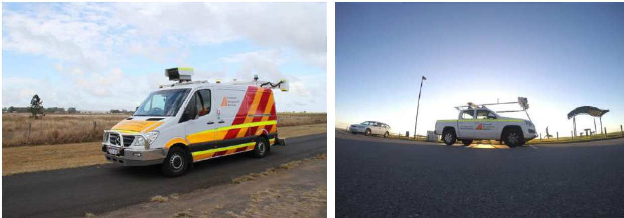
Figure 3. PMS Data Collection Equipment. Sealed Network (left). Unsealed Network (right)
