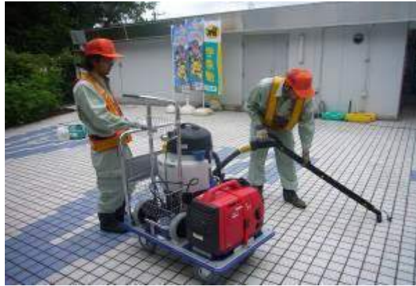
Figure 9: Using the gum removal machine
