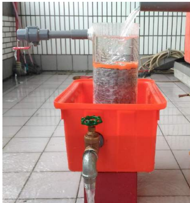
Figure 5. Scheme of constant-head permeability test (Photos taken by Ping-Ni Hou).
