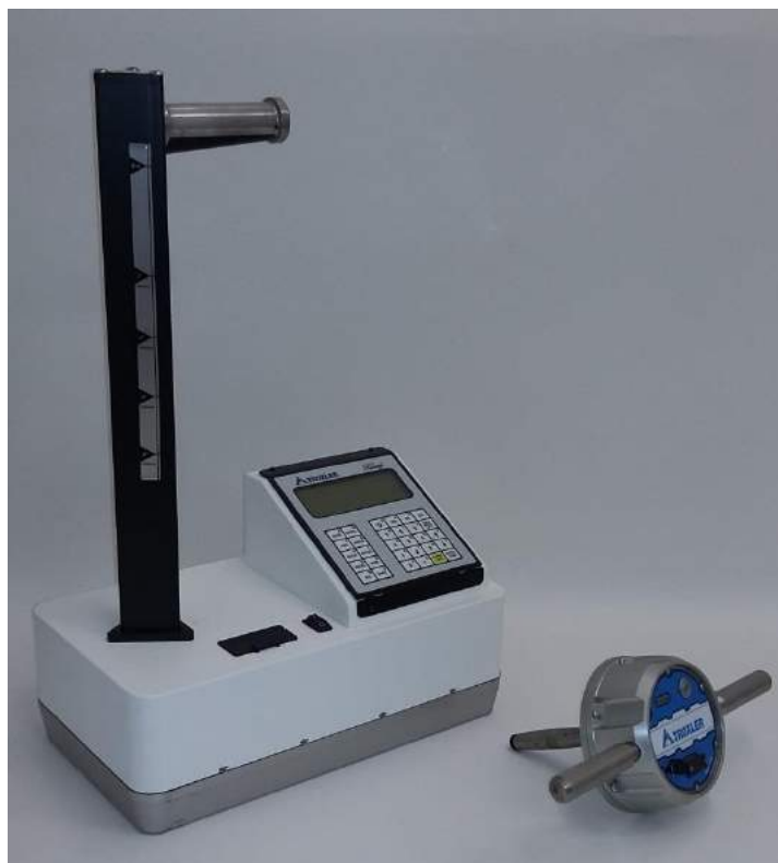
Figure 2. The Low-activity N for soil wet density measurement: Troxler Model 4590 (left) and the non-nuclear moisture probe: Troxler Model 6760 (right). The moisture probe communicates wirelessly with the gauge.
