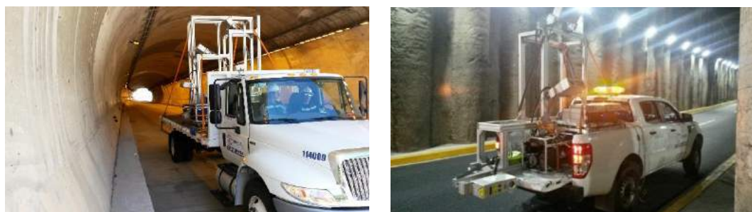
Figure 7 – The Tunnelings system installed on truck with six sensors and on a van with four sensors
