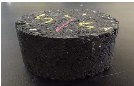
Figure 3. Specimen for deformation strength
