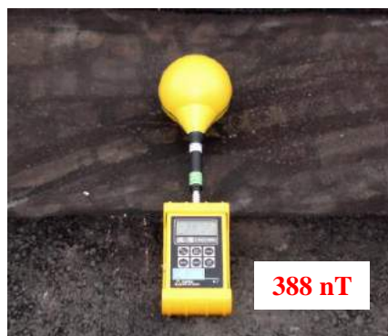
Photo 9. Magnetic field measurements when apart laterally from the coil. (Exposure Level Tester, ELT-400 (Narda), Low frequency 1Hz-400kHz)
