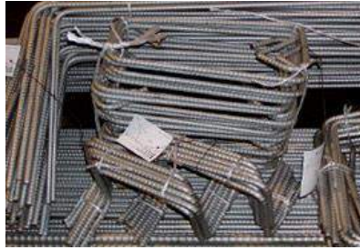
Photo 4. Stainless rebar used for concrete trough.
