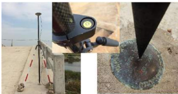
Figure 11. Survey measurement on the DRR survey mark
