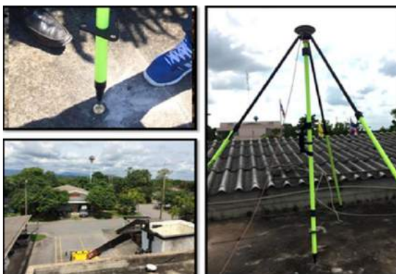
Figure 12. measurement over the new survey mark
