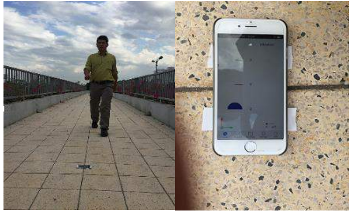
Figure 9 Measurement of vibration using smartphone
