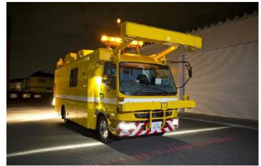
Photo 2: Exterior view of the vehicle in measurement mode Note: Only the 26 red light beams are visible (690 nm @ 200 mm)
