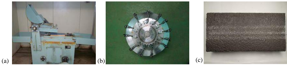
Figure 6. Stripping resistance test (Rebelling test) (a) Overview, (b) Wheel with chain, (c) Specimen after the test.
