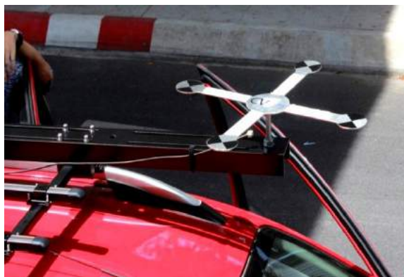
Figure 7. Special apparatus Helico for determination of positioning of the GNSS antenna
