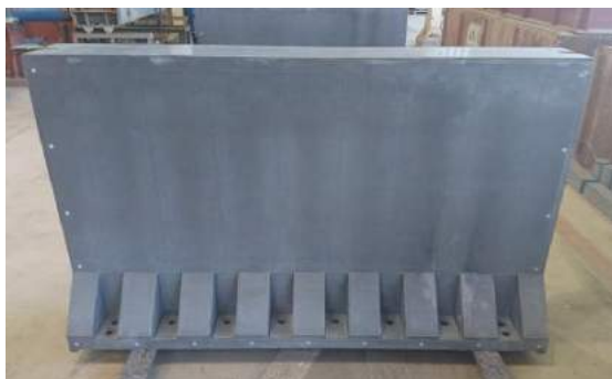
(a) UFC Barrier front surface
