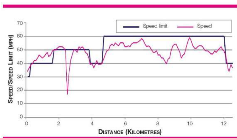
65 Figure 3. Average speeds versus speed limits on a length of UK B class road
