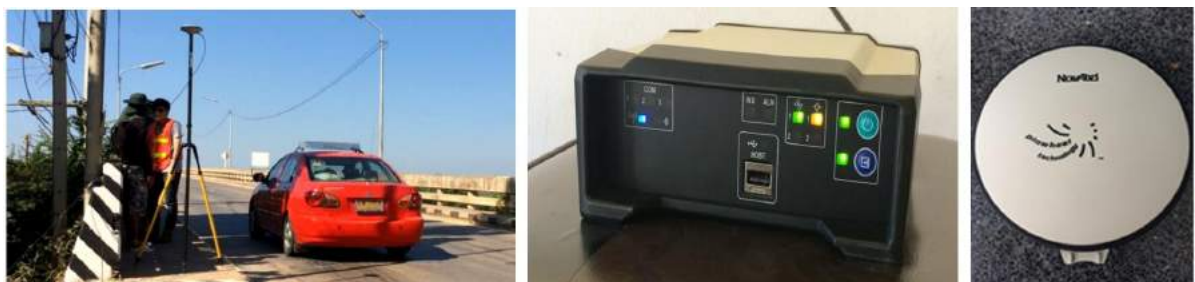
Figure 10. Setup GNSS Base-Station
