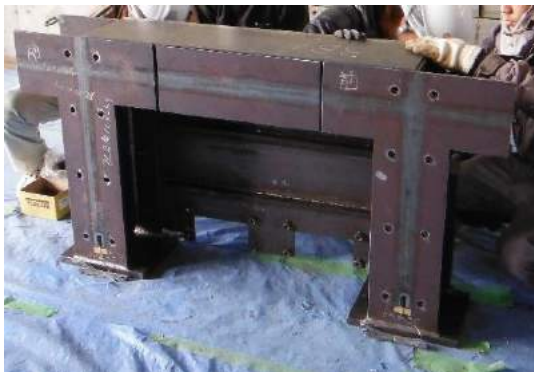
(a) BC Barrier wall provisional assembly
