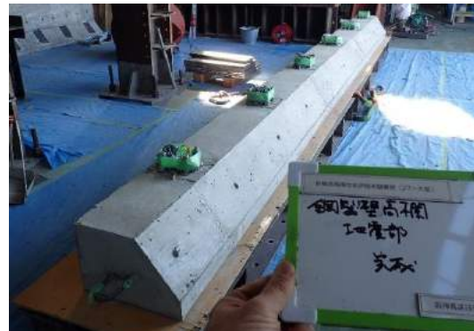
(b) BC Barrier wheel guard concrete part
