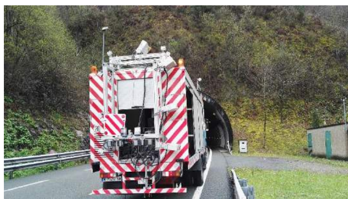
Figure 4 – Subsystems (Lidar-Infrared Visible cameras) assembled together with 3D cameras on a truck
